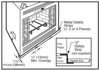
Fig. 14 Safety strip installation.
